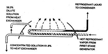
This additional refrigerant vapor (dotted arrows) is produced when dilute solution from the Heat Exchanger is heated by refrigerant vapor from the First Stage Generator. The additional concentrated solution (light grey) that results is returned to the Heat Exchanger. The refrigerant vapor from the First Stage Generator condenses into liquid (dark grey) giving up its heat, and continues to the Condenser.
