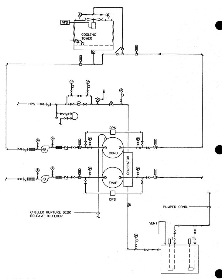
ABSORPTION CHILLER FLOW DIAGRAM
