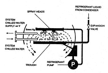
The refrigerant effect cools returning system chilled water in the Evaporator tubes. The refrigerant liquid/vapor picks up the heat of the returning chilled water, cooling it from 54°F to 44°F. The chilled water is then supplied back to the system.
